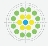
Illustration shows 19 contacts. Same principle of up to 3 levels (external, intermediate, central) applies for all MiniMax configurations. If only 1 level, use External level. If 2 levels, use External and Intermediate levels.
