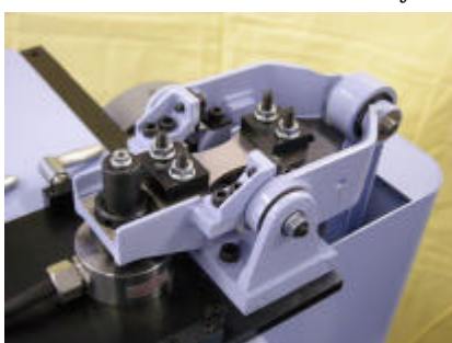
Test force introducing parts and bending moment measuring parts via load cell
